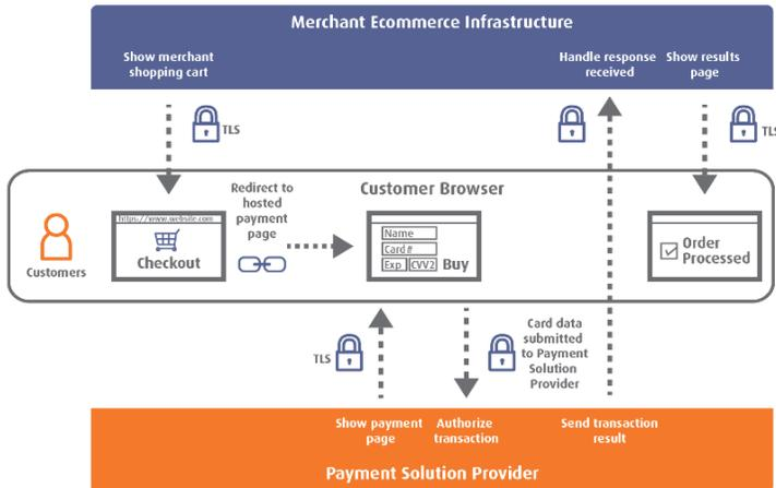
The diagram illustrates the **hosted payment page method**, showing how this method also fulfils the criteria for SAQ A.
